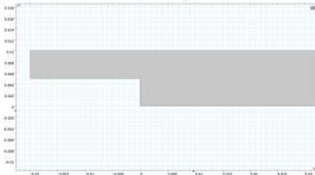
Figure 1. Geometry of an abruptly expanding pipe
